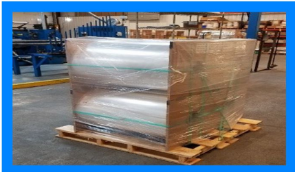
Header Pack – 6" Cores - 22.5" OD - one to four rolls per pallet depending on width and pallet
